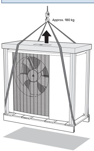
If F2120 needs to be transported across soft ground, such as a lawn, we recommend using a crane truck that can lift it to the installation location. When F2120 is lifted with a crane, the packaging must be untouched.
