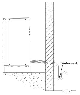
The condensation water is lead to an indoor drain (subject to local rules and regulations).
