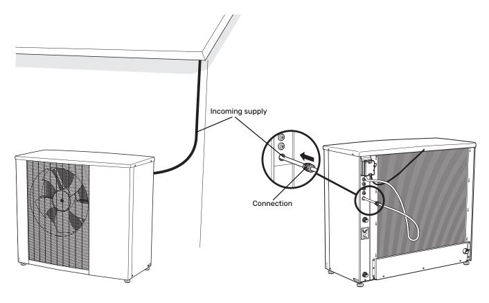
Incoming supply cable is enclosed and factory-connected to terminal block X1. Outside the heat pump there is approx. 1.8 m of cable available. The supply cable should be cut to a suitable length.
