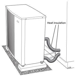
All outdoor pipes must be insulated with at least 19 mm thick pipe insulation.
