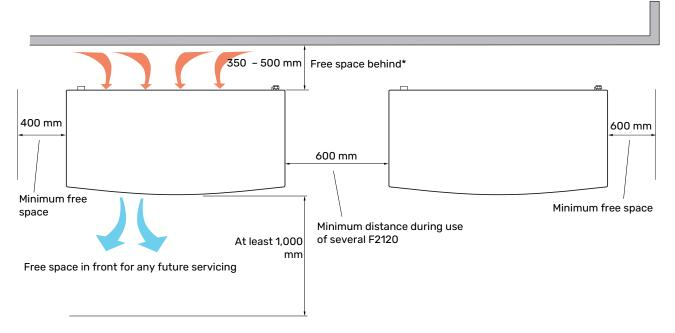
\* The space behind must not exceed 500 mm in locations that are exposed to the wind.
