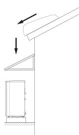
If there is a risk of snow slip from roof, a protective roof or cover must be erected to protect the heat pump, pipes and wiring.
