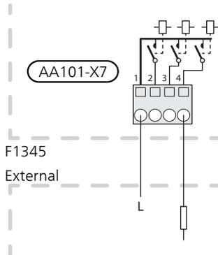
All additional heat can be blocked by connecting a potential-free switch function to AUX input on terminal block AA3-X6 and AA101-X10. The function must be activated in menu 5.4.
