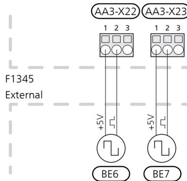
Activate the energy meter(s) in menu 5.2.4 and then set the desired value (energy per pulse) in menu 5.3.21.
