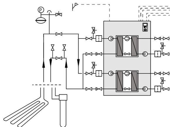
Install the brine pump (GP16) according to the circulation pump manual for connection of incoming brine (EP14-XL6) and (EP15-XL6) between the heat pump and shut-off valve (see image).
