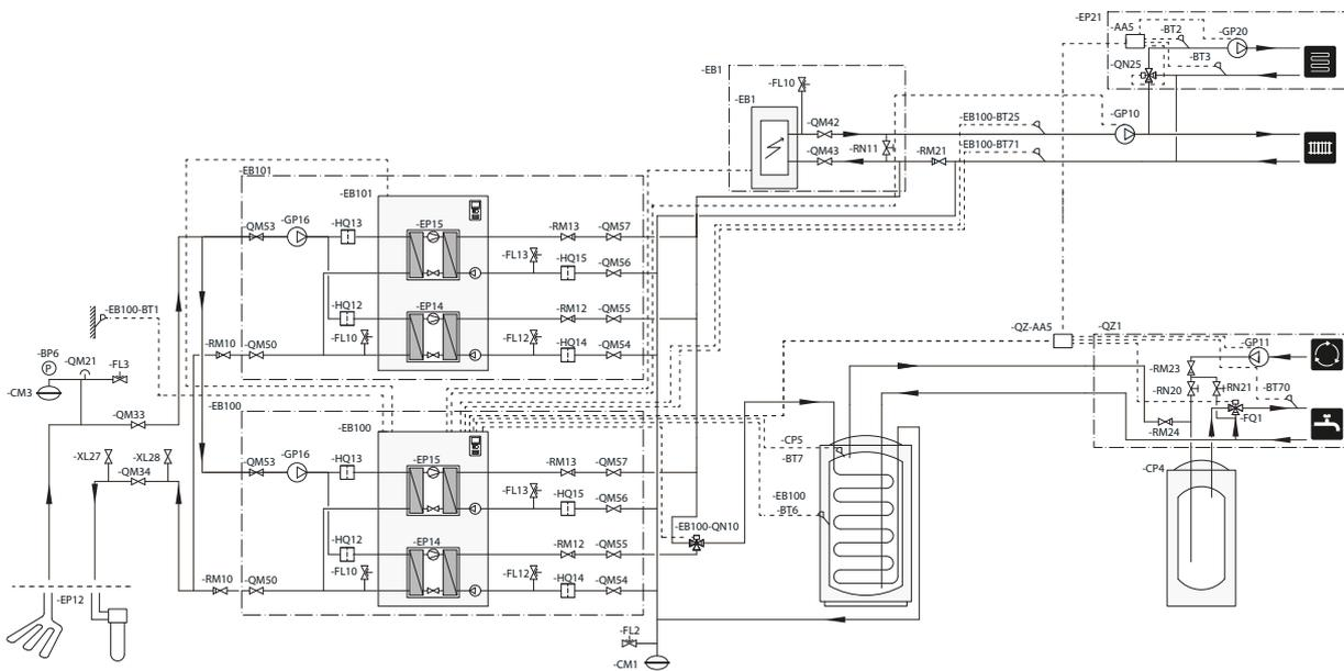
The heat pump (EB100) prioritises charging of hot water with a cooling module (EP14) via a reversing valve (EB100-QN10). When the water heater/accumulator tank (CP5) is fully charged, (EB100-QN10) switches to the heating circuit. When there is a demand for heat, cooling module (EP15) starts in heat pump (EB101) first. In the event of a large demand, cooling module (EP14) also starts in (EB101) for heating operation.
