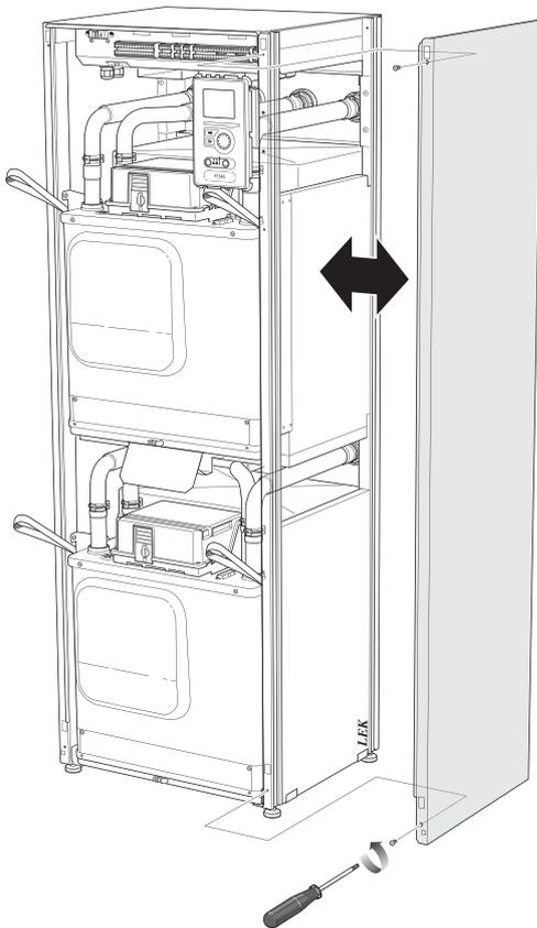
The side covers can be removed to facilitate the installation.
